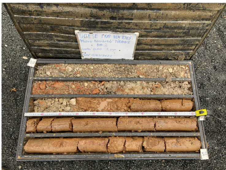
Foto nr.6 Kampionet e marra nga sonda BH-2; thellesia (0.00-5.00)m Photo no.6 Samples taken from BH-2; depth (0.00-5.00)m
