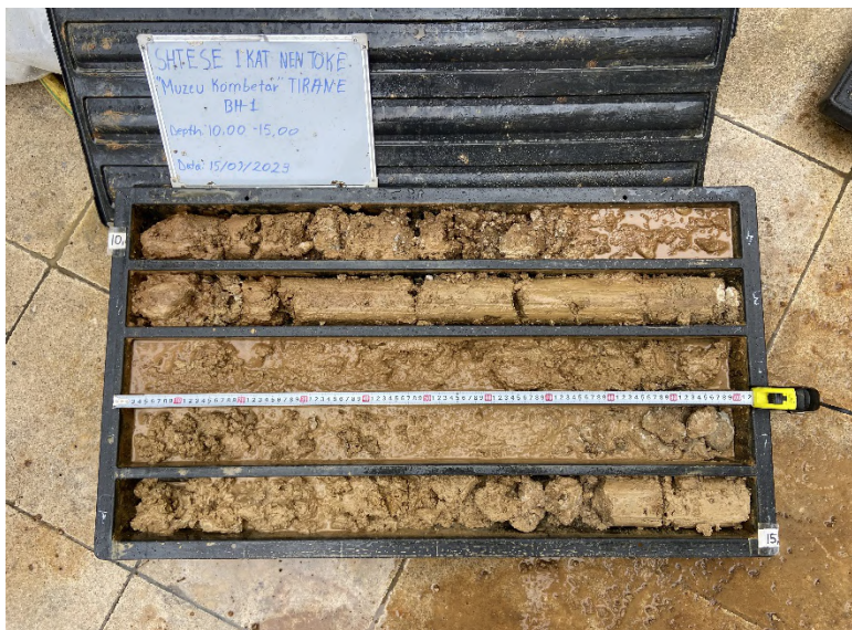
Foto nr.4 Kampionet e marra nga sonda BH-1; thellesia (10.00-15.00)m Photo no.4 Samples taken from BH-1; depth (10.00-15.00)m
