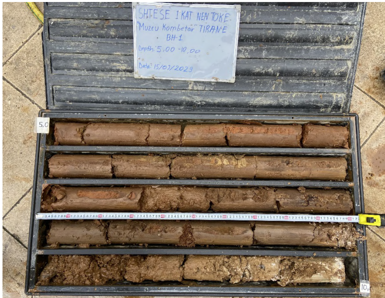
Foto nr.3 Kampionet e marra nga sonda BH-1; thellesia (5.00-10.00)m Photo no.3 Samples taken from BH-1; depth (5.00-10.00)m
