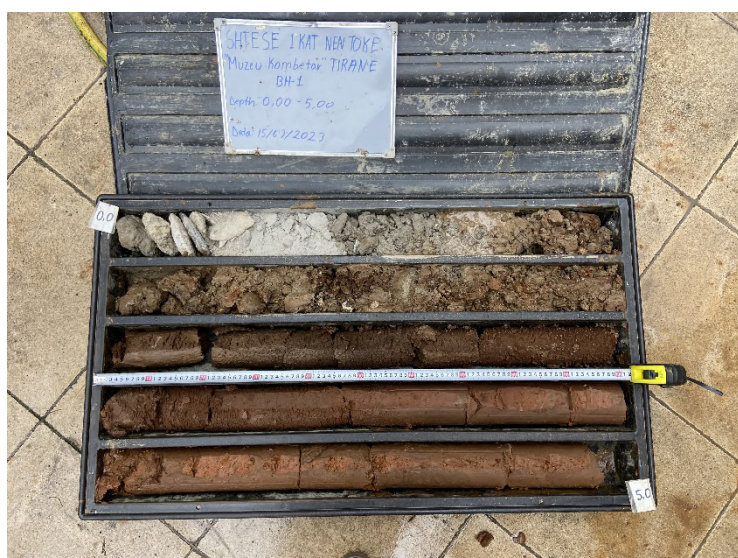
Foto nr.2 Kampionet e marra nga sonda BH-1; thellesia (0.00-5.00)m Photo no.2 Samples taken from BH-1; depth (0.00-5.00)m
