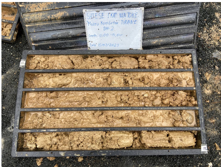
Foto nr.8 Kampionet e marra nga sonda BH-2; thellesia (10.00-15.00)m Photo no.8 Samples taken from BH-2; depth (10.00-15.00)m
