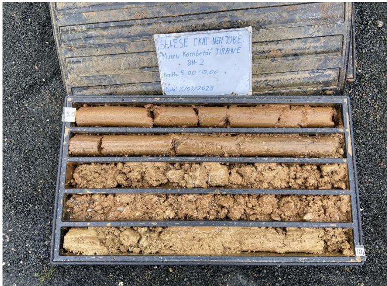
Foto nr.7 Kampionet e marra nga sonda BH-2; thellesia (5.00-10.00)m Photo no.7 Samples taken from BH-2; depth (5.00-10.00)m
