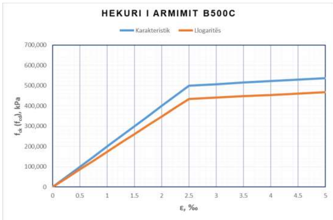
Fig. 4.8: Lakorja sforcim-deformim, B500C
