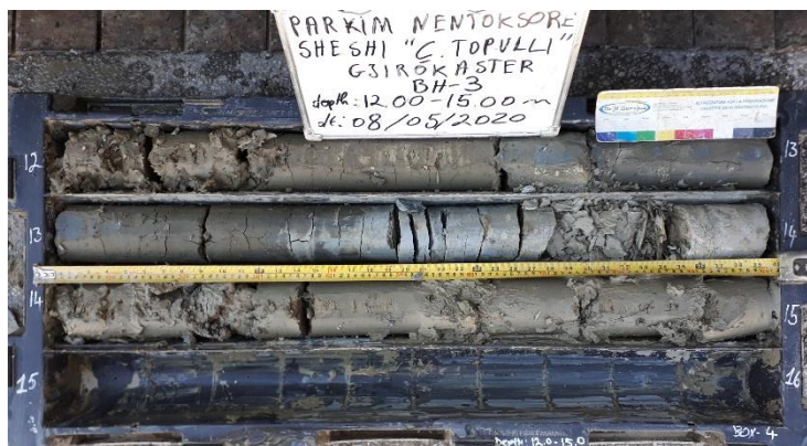
Photo no.5 Samples taken from BH-3; depth (12.0-15.0)m
