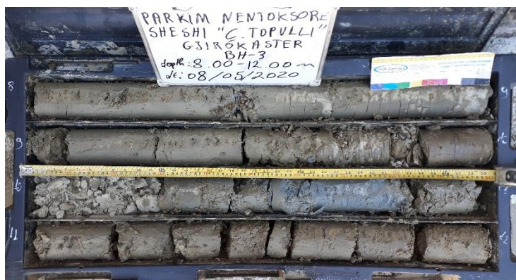
Photo no.4 Samples taken from BH-3; depth (8.0-12.0)m
