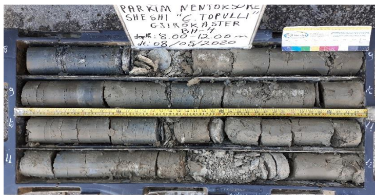
Photo no.4 Samples taken from BH-4; depth (8.0-12.0)m
