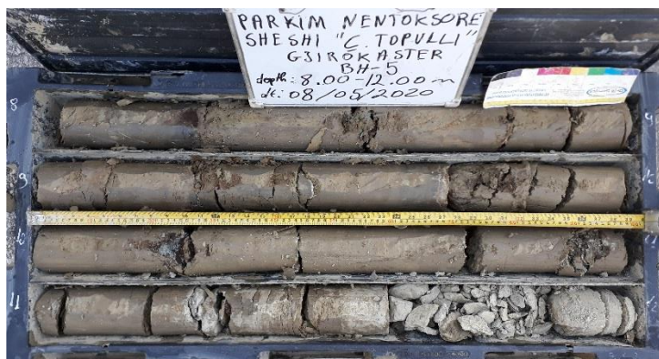
Photo no.4 Samples taken from BH-5; depth (8.0-12.0)m
