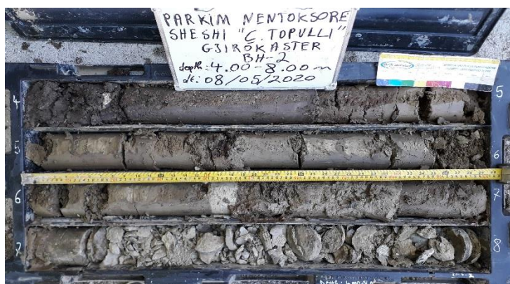
Photo no.3 Samples taken from BH-2; depth (4.0-8.0)m
