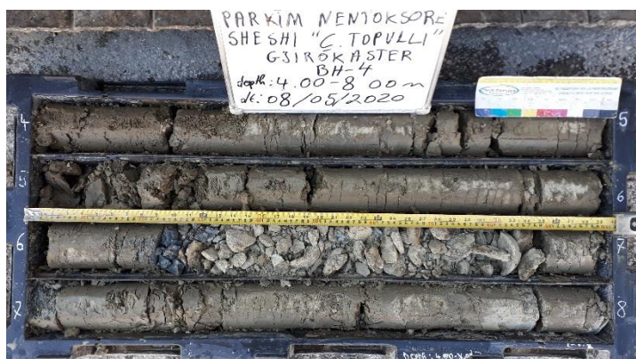
Photo no.3 Samples taken from BH-4; depth (4.0-8.0)m
