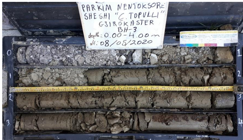
Photo no.2 Samples taken from BH-3; depth (0.0-4.0)m
