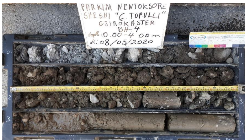
Photo no.2 Samples taken from BH-4; depth (0.0-4.0)m
