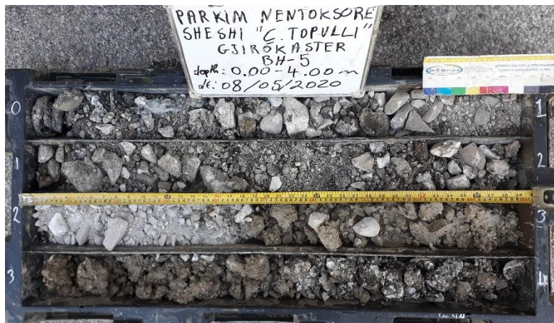
Photo no.2 Samples taken from BH-5; depth (0.0-4.0)m
