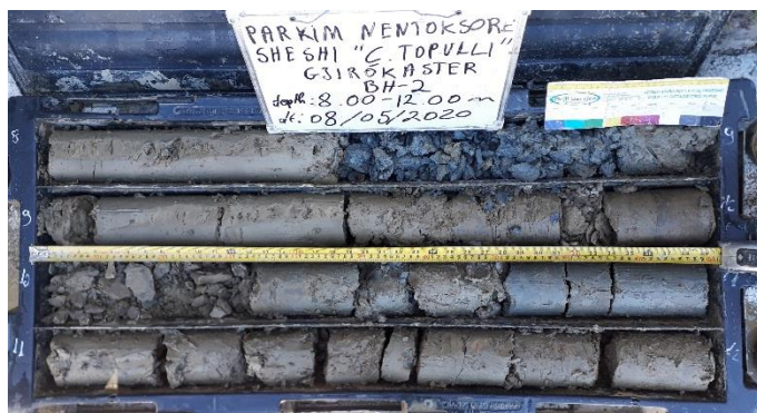
Photo no.4 Samples taken from BH-2; depth (8.0-12.0)m
