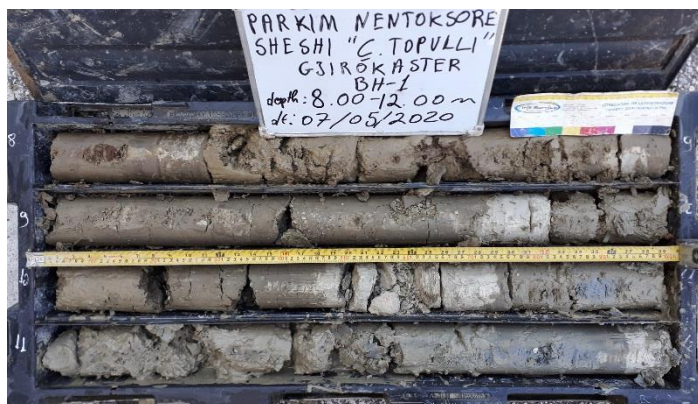
Photo no.4 Samples taken from BH-1; depth (8.0-12.0)m
