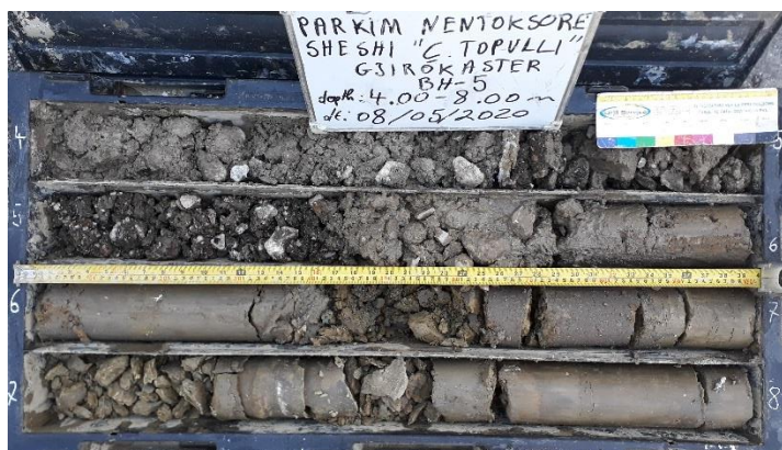
Photo no.3 Samples taken from BH-5; depth (4.0-8.0)m
