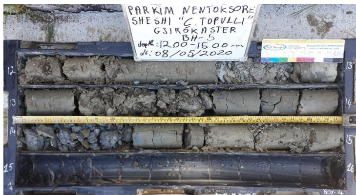
Photo no.5 Samples taken from BH-5; depth (12.0-15.0)m
