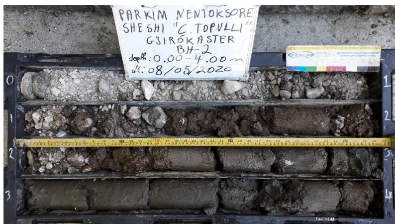
Photo no.2 Samples taken from BH-2; depth (0.0-4.0)m
