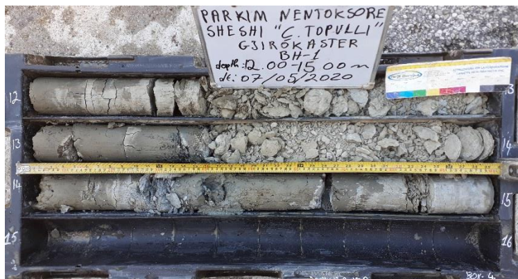
Photo no.5 Samples taken from BH-1; depth (12.0-15.0)m
