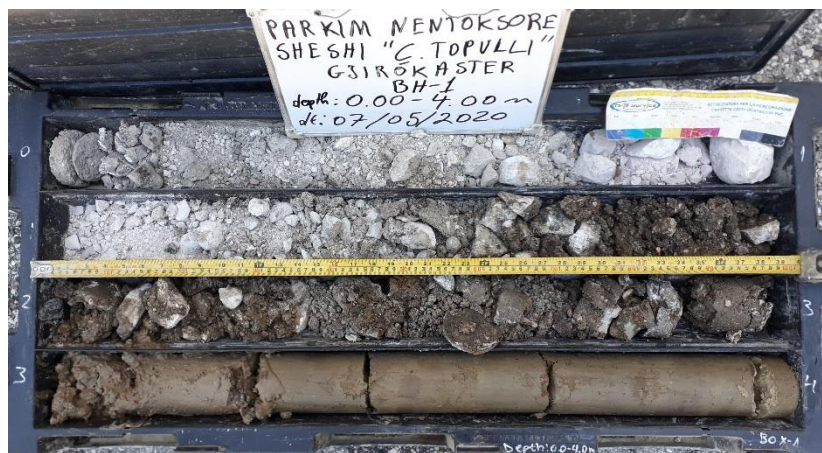
Photo no.2 Samples taken from BH-1; depth (0.0-4.0)m
