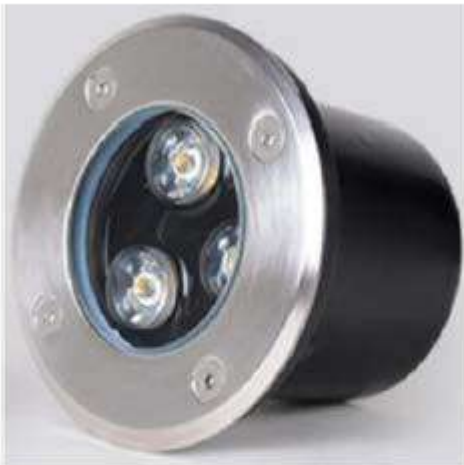
Led underground lamp: DC12V, 6W, 110-120lm/W, 3000K, IP67 and IK10, size: D120*H90mm, inner diameter 62mm, hole size: 115mm, 3pc CREE led, stainless cover+aluminum alloy shell+tempered glass, 3 year warranty.
