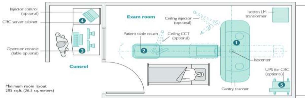
This layout represents minimum space for equipment installation and service access.
