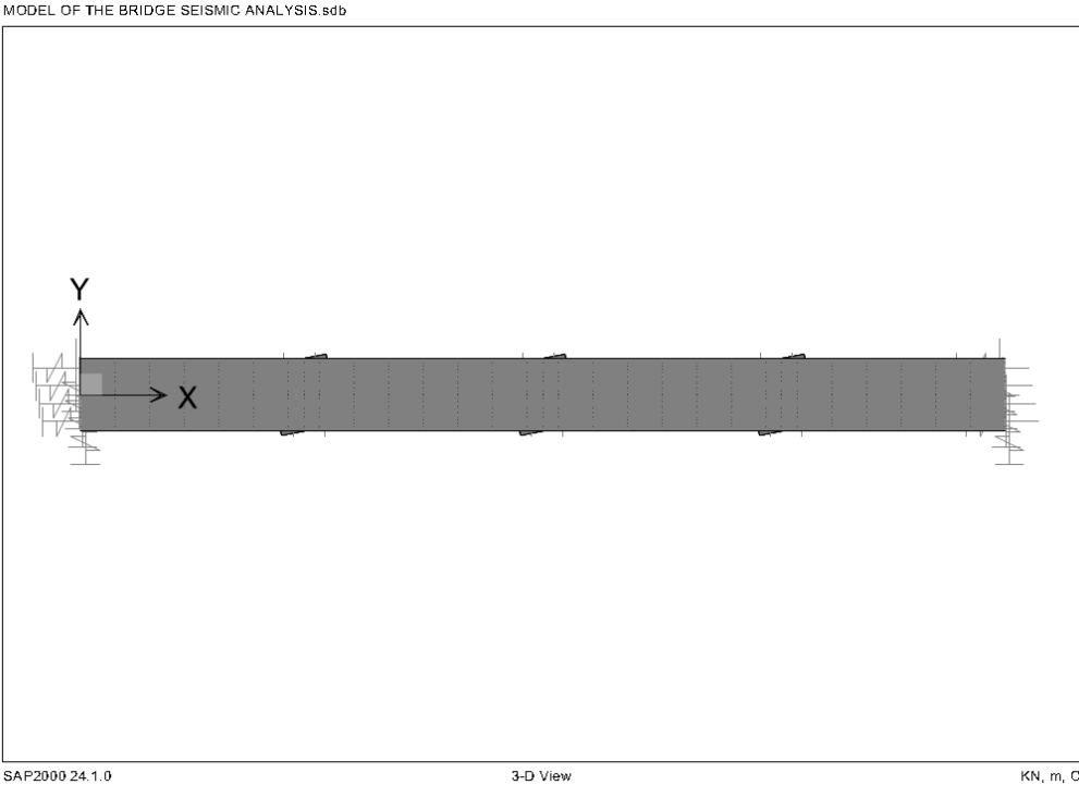
Figure 6-3 Plan-view Model-Superstructure and Piers
