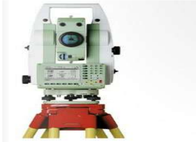
Fig.4 Total Station Leica 1200+
